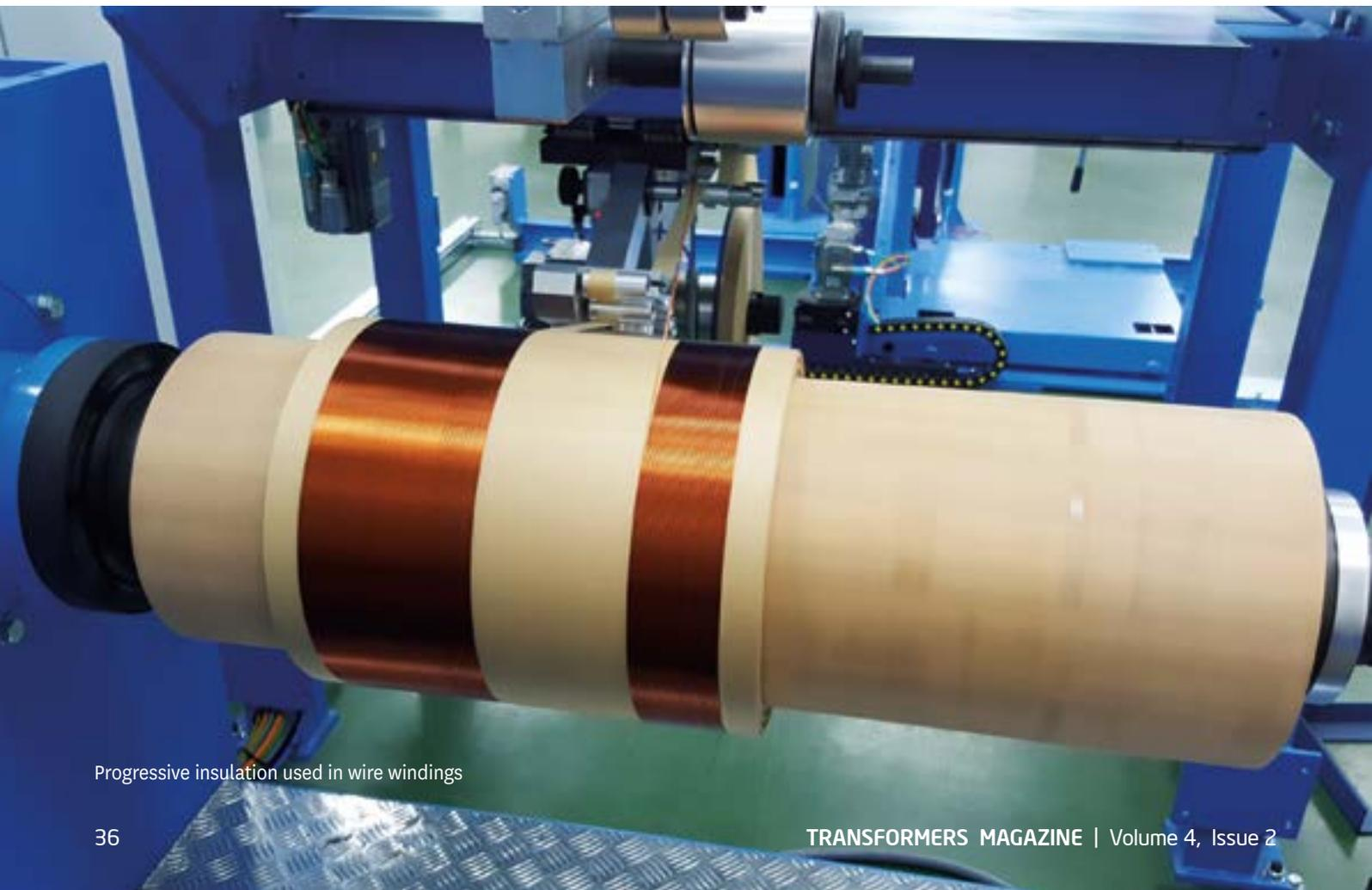
Progressive insulation used in wire windings
